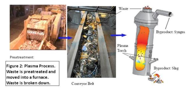
As shown in Figure 2, waste first enters the system by a conveyor belt. Pretreatment is optional. If waste is appropriately sorted into categories i.e. by metallic or organic material; and
